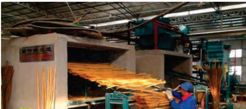
Figure 2.2. 3Drying Bamboo Silver using dryer machine
