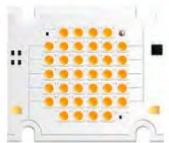
LED based light engine module
