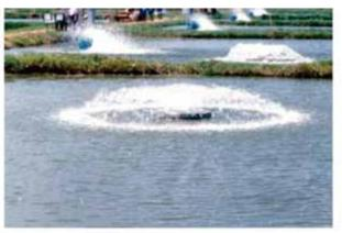
Fig 3.3.1 paddlewheel aerator airbolwer
