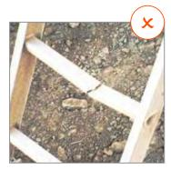
Fig. 3.2.5. Cracks in ladder
