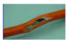
Fig. 3.2.28. Worn insulation around wire
