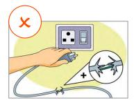
Fig. 3.2.2. Torn electric cable
