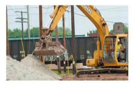
Fig. 3.2.35. Unsafe ovehead power lines
