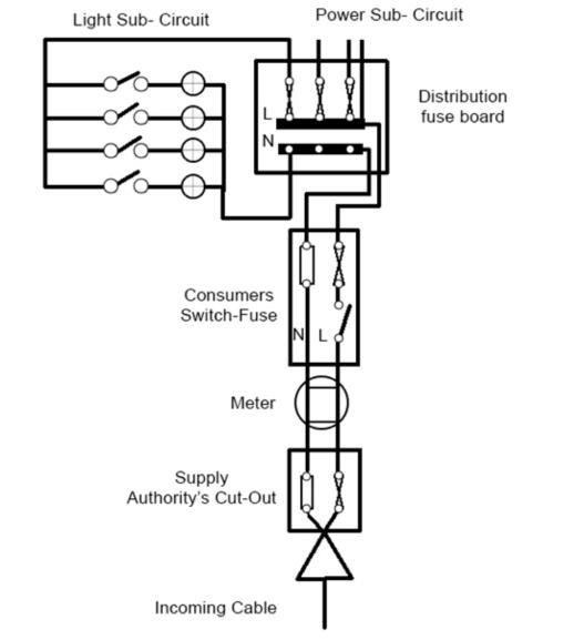
Fig. 1.4.15. Single phase installation
