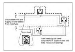
Fig. 9.1.3. Final ring circuit conductor continuity test
