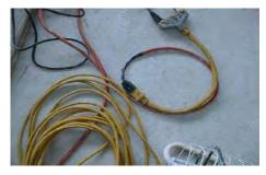
Fig. 3.2.27. Wires joined improperly
