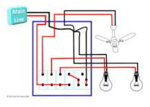
Fig. 8.1.1 . Connecting distribution panel with main board
