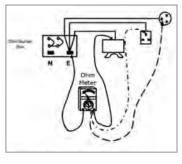
*Fig. 9.1.2. Protection Conductor Continuity Test*
