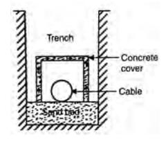
Fig. 6.1.1. Direct Laying Method
