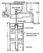
Fig. 7.2.3. Procedure for Pipe Earthing
