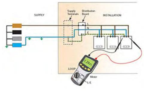
Fig. 7.2.4. Process for Measuring Ground Resistance Using an Ohmmeter
