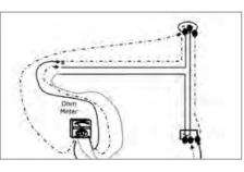
Fig. 9.1.4. Live and neutral conductor continuity test
