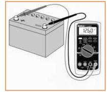
Fig: 2.3.4: Battery Attached to Multi Meter
