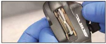
*Fig: 2.3.15.3 Changing Hydraulic Disc Brake Pads*
