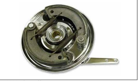
Fig: 2.3.2.9 Brake Assembly
