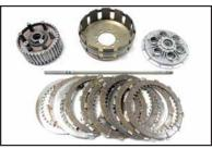
Fig: 2.3.8.1 Different Parts of Clutch Assembly
