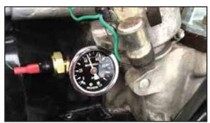
Fig: 2.3.19.1 Gauge to Check Oil Pressure
