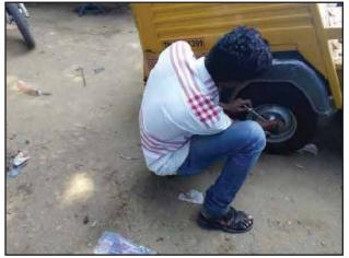
Fig: 2.3.13 Dismantling & Assembling of Wheels
