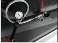
Now we connect the battery voltage. The purge valve clicks and the vacuum immediately drops. This purge valve is good.
