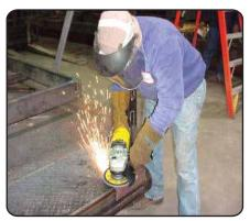
Fig: 5.2.3.9 Wear Safety Glasses While using a Grinder
