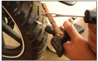
Fig: 2.3.13.2 Repairing Punctured Tyre
