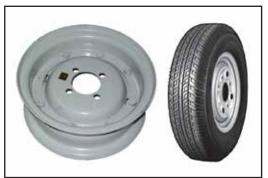
Fig: 2.3.2.20 Rims and Tyres of a Three Wheeler
