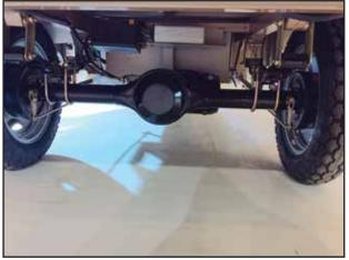
Fig: 2.3.9.3 Rear Axle of a Three Wheeler
