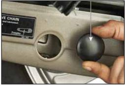
Fig. 2.3.17 Servicing Drive Chain of Motorcycle
