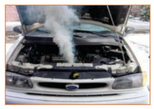
Fig 2.2.34 Overheated Engine
