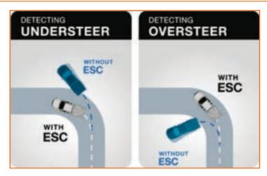
Fig 2.2.4 Electronic Stability Control
