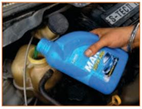
Fig 2.2.21 Filling the Radiator Coolant Oil
