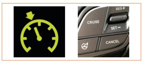
Fig 2.2.2 Cruise Control Dashboard Lamp and Dashboard Button
