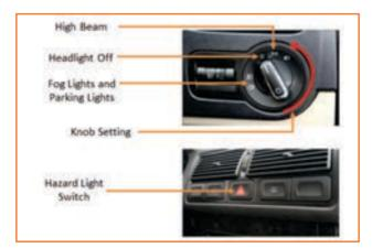
Fig 4.3.4 Light Controls on the Dashboard
