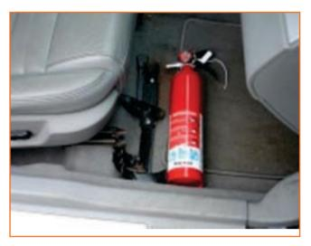
Fig 8.5.4 Fire-Extinguisher in a Vehicle
