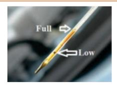
Insert the dipstick back into the tube.
