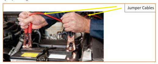
Fig 2.2.32 Mechanic Jump Starting a Car
