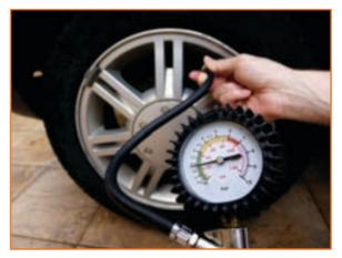
Fig 2.2.15 Using an Air Gauge to Measure Tire Pressure
