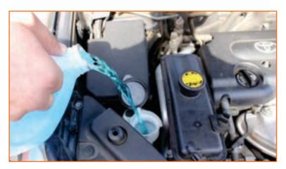
Fig 2.2.25 Filling the Wiper Fluid
