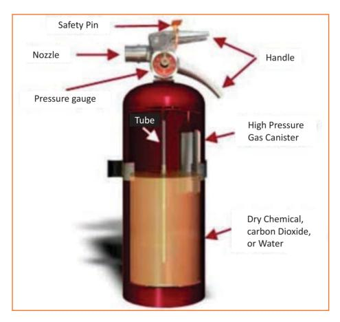
Fig 8.5.1 Parts of a Fire Extinguisher
