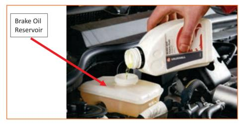
Fig 2.2.23 Filling the Brake oil Reservoir
