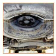
Vehicle undercarriage before removal of rust
