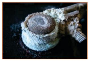
Fig 2.2.31 Battery Corrsion at terminals
