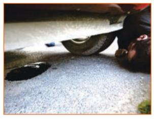
Fig 2.2.12 Checking for Engine Oil Leakage
