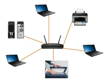
Fig. 1.5.1: Basic layout of a network
