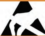
A triangle with a hand that is crossed out is the symbol used to represent a product that is sensitive to electrostatic discharge (ESD).
