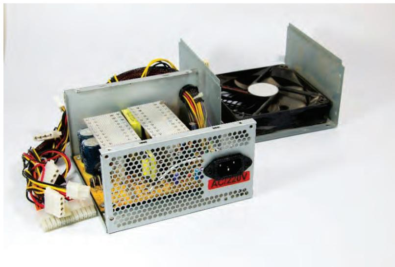
*Fig. 2.2.3: Interior view of a PSU*
