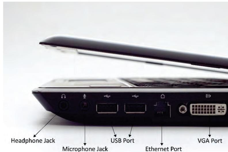
*Fig. 3.1.11: Different connection ports in a laptop computer*
