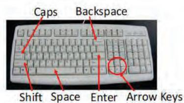
Fig.8.2.2 Parts of a Keyboard
