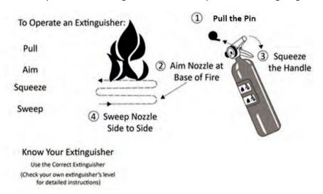
Fig 2.2.1: Fire extinguisher operation
