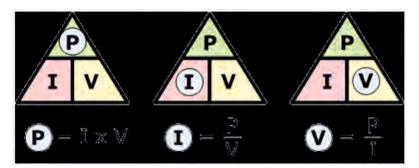
Fig 1.1.4: Formulae for calculating power
