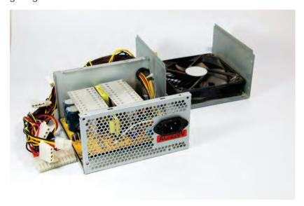
Fig. 2.23: Interior view of a PSU
