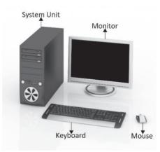
Fig. 1.1.16: A desktop computer along with its CPU and peripherals
