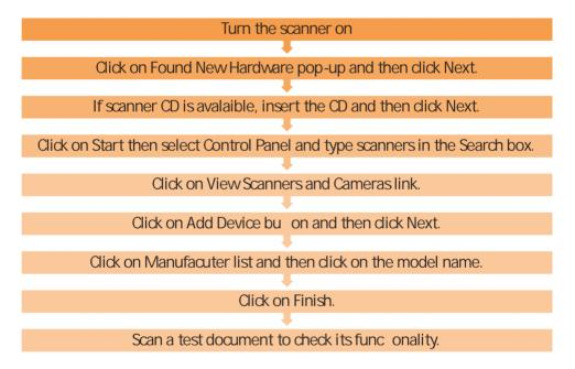
Fig. 3.2.3: Steps to install a scanner
