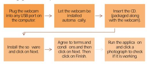
Fig. 3.25: Steps to install a webcam
