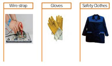
Fig. 6.3.3: Safety gears for preven on from ESD
