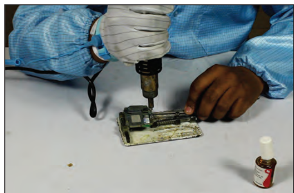
Fig: 3.3.7.1.2 Soldering Flux on Charging Connector
