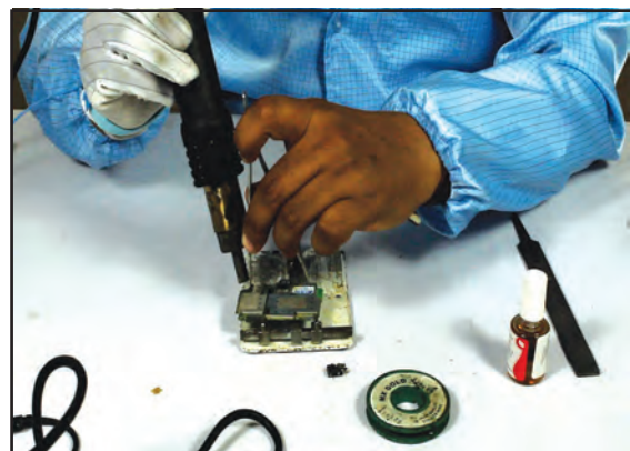
Fig: 3.3.7.3.3 Headphone Connector Soldering - Step 2
