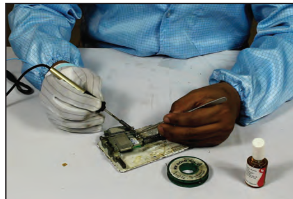
Fig: 3.3.7.1.5 Charging Connector Soldering - Step 2
