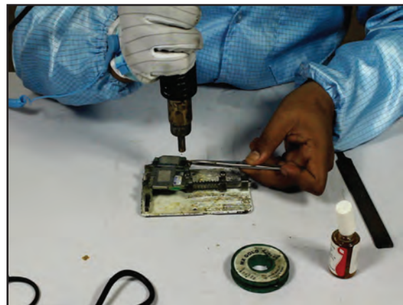
Fig: 3.3.7.3.2 Headphone Connector Soldering - Step 1
