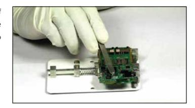
Step 3: Fisrt apply flux using tweezers on the component we need to remove. Now switch On hot airgun and place it above the component exactly at 90 degree. Now we can see this component can be separated easily from the motherboard. Remove the ceramic capacitor and keep it in safe place. Now Switch Off the hot air gun.
