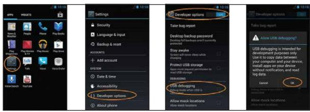
Fig: 3.3.21.1.2 USB Debugging Mode -Android 3.0 - 4.1 X
