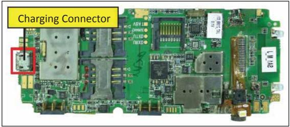
Fig: 3.3.7.1.1 Motherboard - Charging Connector
