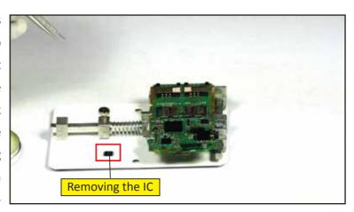
Step 5: Now inorder to place the IC back, we will apply flux and with the help of soldering gun try to do the re-soldering. At first we will clean all the legs then after apply flux on IC base and clean it properly.
