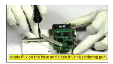
**Step 6:** Now we have assembled ceramic capacitor properly to its location using hot air gun. This is called soldering and De-soldering process.
