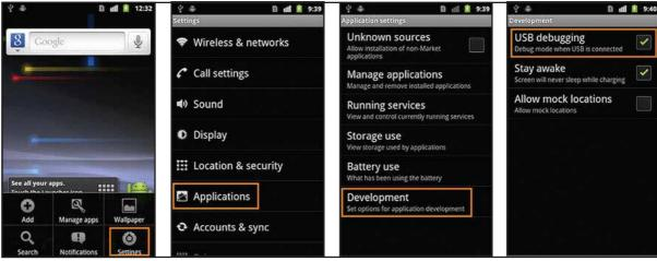
Fig: 3.3.21.1.1 USB Debugging Mode -Android 2.0 - 2.3X
