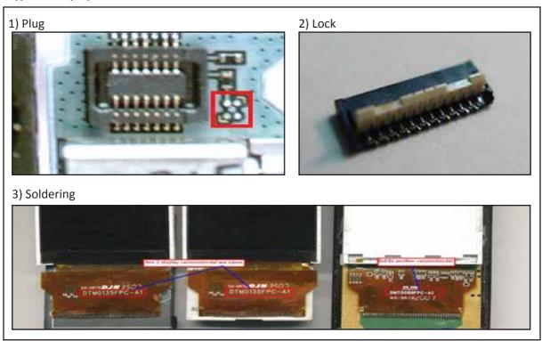
Fig: 3.3.8.7 Display Connector Type
