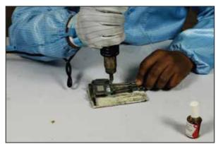
Fig: 3.3.7.1.2 Soldering Flux on Charging Connector
