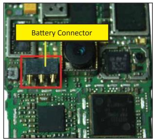
Fig: 3.3.7.2 Battery Connector
