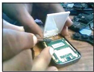
Fig: 3.3.7.9.2 Display Strip Assembly
