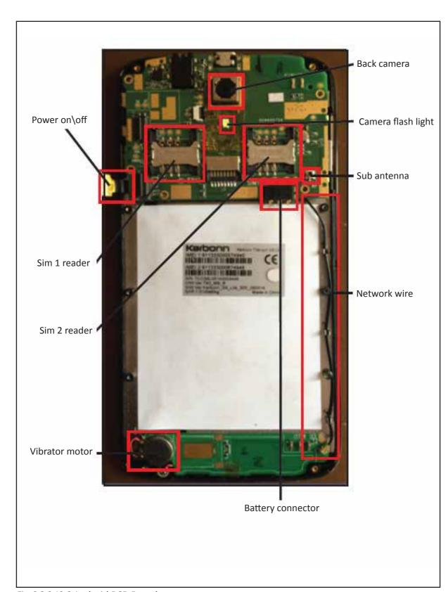
Fig: 3.3.8.13.6 Android PCB Board
