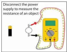
Fig: 3.3.10 Measuring Resistance
