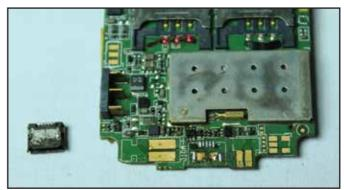
Fig 3.5.7.1.3: Charging Connector and Slot
