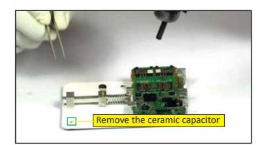
Step 5: This is the base from where we can remove ceramic capacitor, apply flux on the base and clean it using soldering gun. Now we have to place the ceramic capacitor back to it's location. Point the hot air gun to the location where we have to place the ceramic capacitor.
