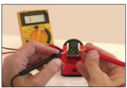
Fig: 3.3.10.4.2 Testing of Mic.
