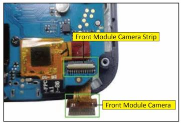
Fig: 3.3.5.7 Front Module Camera
