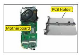
**Step 12:** Now remove speaker and ringer form motherboard. First remove vibrator using hot air gun and same way we will remove vibrator
