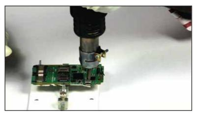
Step 4: Now you can see we have remove this charging socket from PCB. This is the lower portion of charging base where it is getting soldered.
