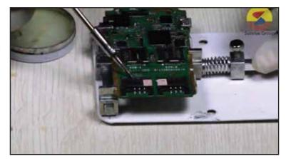
Step 5: Now we will use another end of jumpering wire to connect broken track. You can see silver base on this track. We will clean the base with the help of solder gun and then apply flux to do the soldering of another end of the jumpering wire. Here we can see we how we did the jumpering from SIM tray pin to base of track. This process is called jumpering
