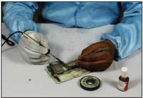
Fig: 3.3.7.1.5 Charging Connector Soldering - Step 2
