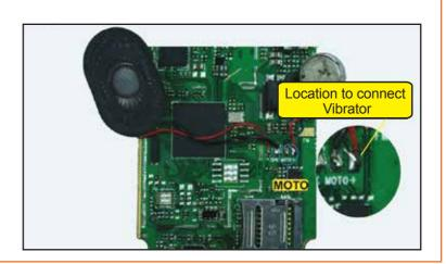
Step 25: Be careful while soldering the wire, always connect positive wire with positive pin and negative wire with negative pin. Location for positive is marked with "+" where as negative is marked with "-" sign.
