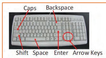
Fig.10.2.2: Parts of a Keyboard
