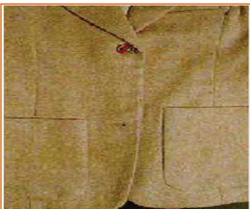
Fig.3.1.9: Fusing distortion
