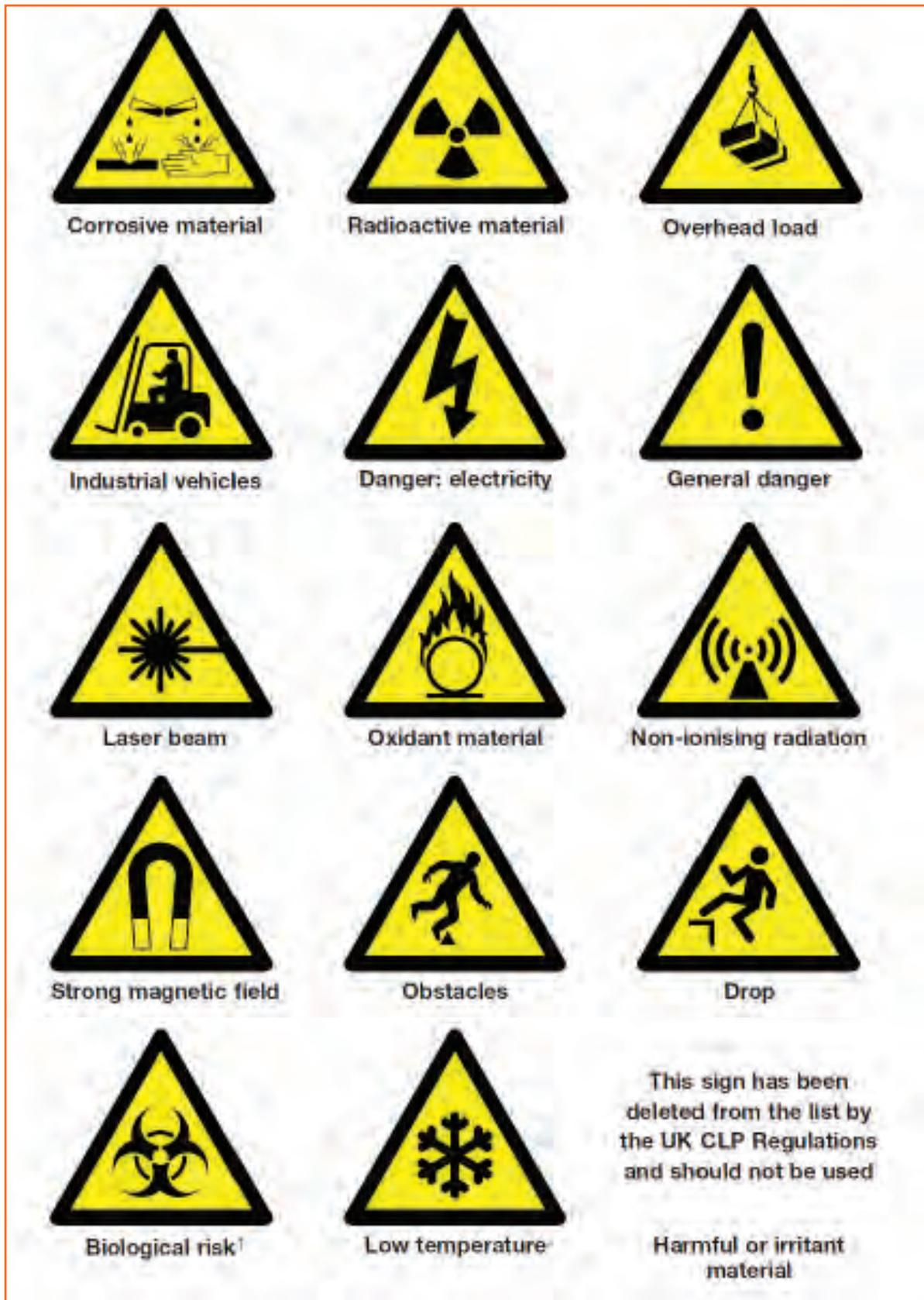
Fig.4.1.14(b): Chemical, Biohazard and Hazardous Material Signs
