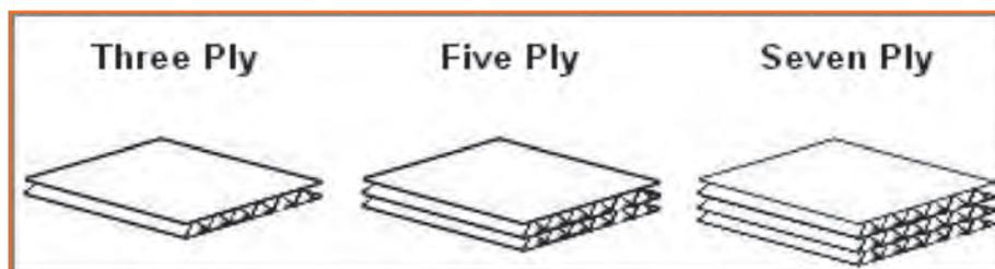
Fig.2.5.9: Deferent types of plies of cartons
