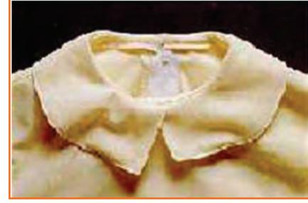
Fig.3.1.6(c): Interlining shrinking
