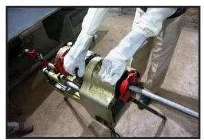
Fig-2.3.33 Pipe threading using Pipe Threading Machine
