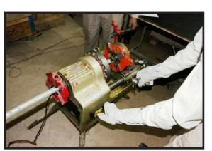
Fig-2.3.34 Pipe threading using Pipe Threading Machine
