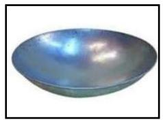
Fig-2.1.47 Mortar Pan
