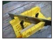
Fig-2.3.29 Cutting pipe with Hexa
