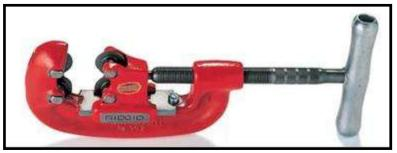
Fig-2.3.28 Pipe Cutting Tool
