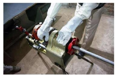
Fig-PG-0130 Pipe Threading Using Pipe Threading Machine
