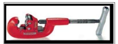
Fig-PG-0023 Pipe Cutter
