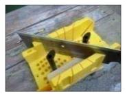
Fig-PG-0126 Cutting pipe with Hexa
