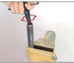
Fig-PG-0029 Reaming The Cut
