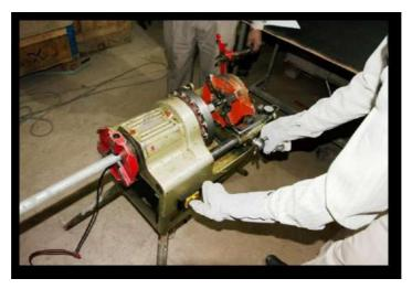
Fig-PG-0131 Pipe Threading Using Pipe Threading Machine
