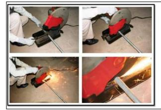
Fig-PG-0127 Pipe cutting with wheel cutters
