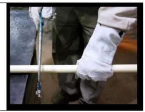
Fig-PG-0128 Pipe cutting using Hacksaws
