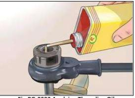
Fig-PG-0033 Applying Threading Oil
