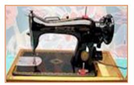
Fig.3.1.1: Hand driven Lockstitch sewing machine
