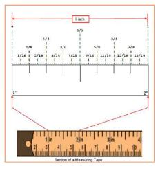
Fig.2.4.6: Fractions in a Measuring tape
