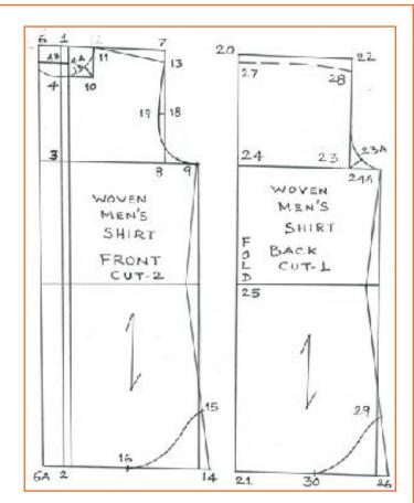
Fig.2.6.1: Drafting of front and back part
