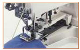
Fig.3.1.5: Button Attachment Machine
