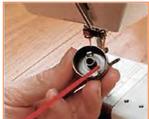
Fig 5.1.2: Cleaning the bobbin and case
