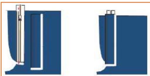
**Step 6:** Take the fly supportive part. Place the zipper with slider facing up on the fly supportive part. Properly align the zipper end and the overlock side of the fly supportive part.
