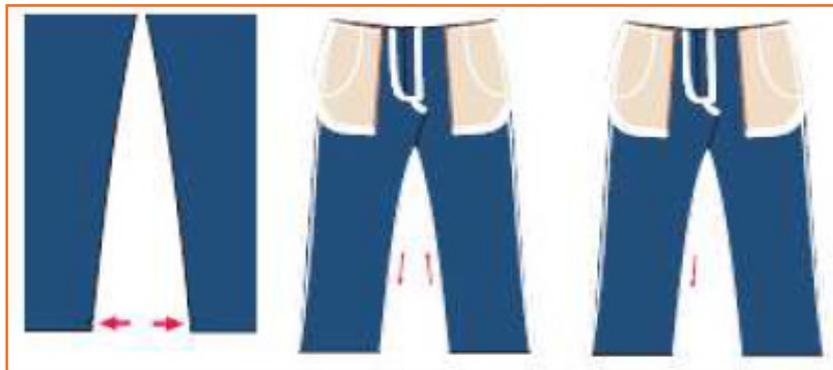
**Step 3:** Put 5-thread overlock stitches starting from bottom to finish at other bottom side.
