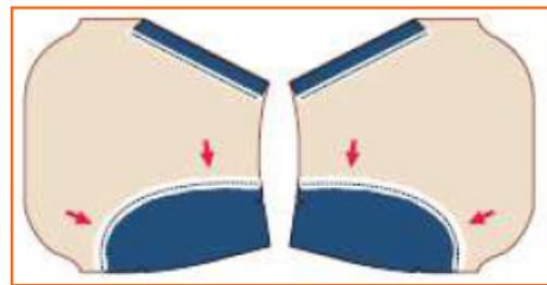
**Step 6:** Put the lockstitch at the edge of the overlock curved stitch.
