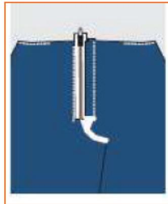
**Step 11:** Leave a gap of 1 mm between the zipper teeth and the edge of the fabric and put top-stitch.
