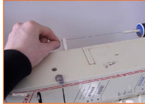
**Step 2:** Allow the string to unwind and put it through this hoop. Mine can also snap in from the back but usually with older machines this is a hoop.
