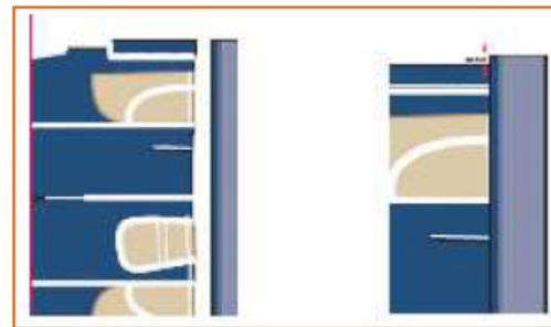
**Step 2:** Place the belt piece, with the folded side up on the backside of the right front. Belt band should be extended by  $\frac{1}{2}$  inch.
