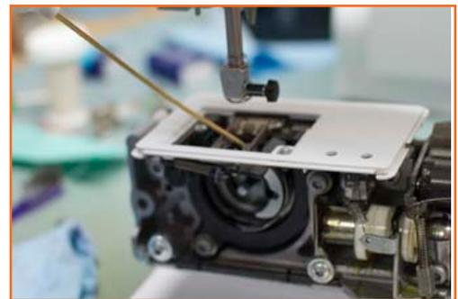
**Step 2:** **Check feed dogs:** Remove the feed dog, clean the feed dogs. Try to pass a rag under them and with an old needle or narrow tool, remove the lint inside the feed channels. Put back the needle plate. If your machine is equipped with a FEED DROP, be sure the feeds are set at UP position. By turning the hand wheel (towards you), check to see if the feeds make their movement.
