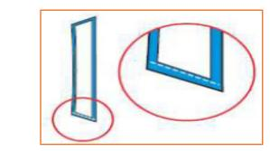
Step 5: Start stitching at a gap of 1 mm from the fusing material from the collar base side.
