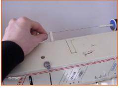
Step 2: Allow the string to unwind and put it through this hoop. Mine can also snap in from the back but usually with older machines this is a hoop.
