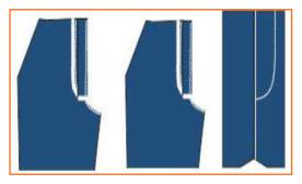
**Step 19:** Turn the piece so that the front side of the fabric is facing up. Put an edge stitch on front rise starting from bottom till the end of J-stitch.
