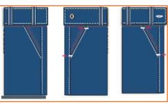
Step 1: Put bartack as per design requirement. Normally bartacks are put at both ends of left and right front pocket mouth and at the end of the front and back pocket joints.
