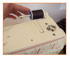
Step 1: This is where the thread goes. If you have a cap or stopper put it on after you put the thread on. Also put the side of the thread with the little cut to the back or bottom.
