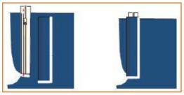
**Step 6:** Take the fl y supportive part. Place the zipper with slider facing up on the fly supportive part. Properly align the zipper end and the overlock side of the fly supportive part.
