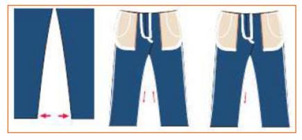
**Step 3:** Put 5-thread overlock stitches starting from bottom to finish at other bottom side.
