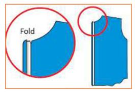
Step 3: Now, fold the fabric 1.5 cm till the first notch mark and press the folded part with an iron.
