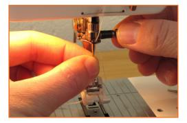
Step 4: Use your fingers initially and then your tool of choice to tighten the needle clamp screw. The tighter you can make this, the better. A loose clamp may leave the needle down in the fabric you are sewing.
