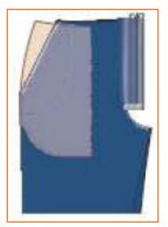
**Step 18:** Reverse the fabric and put 6 mm stitch on the curved portion of the front rise.
