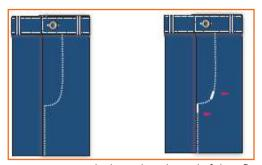
**Step 2:** Put the bartack at the end of the J-fly and at the curve of the J-fly.
