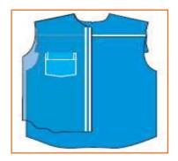
**Step 2:** The alignment should be such that the right side of the outer yoke piece faces the right side of the back piece of the shirt.
