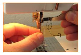
Step 1: Hold the needle with your left hand and undo the screw at the top of the needle with your right hand.
