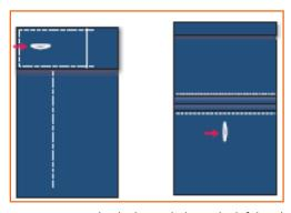
Step 1: Make the buttonhole on the left hand side belt as per design requirement. Make another buttonhole on the back pocket.
