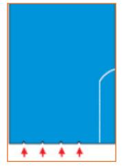
Step 1: First, check that there are 4 notches for sleeve pleatsand one notch at the centre of sleeve bottom.
