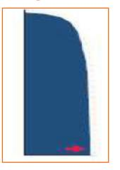
Step 1: Take the fused J-fly piece and put overlock stitch on the face side of the fabric starting from bottom of the curved side till the top.
