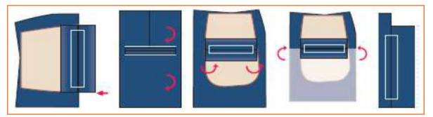
**Step 15:** Put overlock stitch at the loose end of the bottom bone piece.
