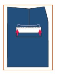
Step 5: Now put a 6 mm stitch starting from back rise side towards the side seam side. The first stitch should be at the notch mark side. Put back tack, both at the beginning and end of the stitch.
