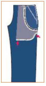
**Step 7:** Put 5 thread overlock stitches on the curved portion of the pocket bag.
