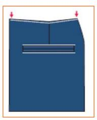
Step 23: Put 3 mm lockstitch at the waistline, starting from the left towards the right, to stitch the loose top end of the pocket bag with the fabric. Fly Making and Attaching
