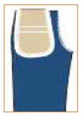
**Step 3:** Now put overlock stitches at the back rise starting from top to bottom.
