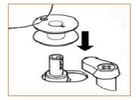
Step 2: Pass thread end, from inside, through small hole in rim of bobbin
