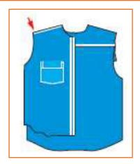
**Step 3:** The pieces are stitched at a distance of 1 cm from the edge leaving the bottom-most ply of the yoke.
