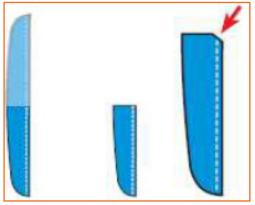
**Step 3:** Fold the neckband and cut a notch at the centre of the upper side.
