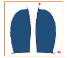
Step 2: Take both the lower facing pieces and put overlock stitch on the curved sides. Again, make sure that the face side of the pieces are on the top.
