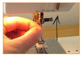
Step 3: With the flat side towards the back, push the new needle up inside the needle clamp as high as it will go.
