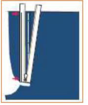
Step 3:Put an edge stitch on the left side of<br/>the zipper from top to bottom.Step 4:Close the zipper and turn the piece<br/>1800 clockwise.
