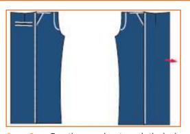
Step 3: Turn the raw edges towards the back. Put topstitches at the edge starting from top to bottom for the right side and bottom to top for the left side.
