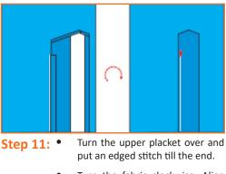
• Turn the fabric clockwise. Align the upper and lower plackets.
