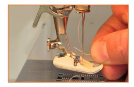
**Step 5:** Re-thread your needle, pushing the thread from front to back.
