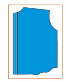
**Step 7:** Again from the bottom, stitch the outer side of the placket using edge stitch.
