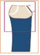
Step 3: Put 6 mm stitch taking ¼ line on throat plate as guide, starting from the top to bottom.
