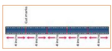
**Step 4:** Put the marking on the strap for the required length.
