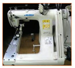
Fig 2.2.37(a): Feed of Arm Machine
