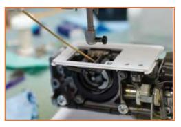
Step 2: Check feed dogs: Remove the feed dog, clean the feed dogs. Try to pass a rag under them and with an old needle or narrow tool, remove the lint inside the feed channels. Put back the needle plate. If your machine is equipped with a FEED DROP, be sure the feeds are set at UP position. By turning the hand wheel (towards you), check to see if the feeds make their movement.
