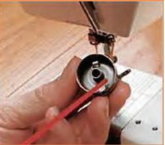
Fig 4.1.2: Cleaning the bobbin and case
