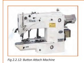
**Button Attach Machine:** Clothes are held together by buttons, a button is one of the most basic elements of fashion. Button sewing work requires a machine, which provides flexibility (in terms of button design, fabric variation, thread thickness etc.) as well as a consistently good sewing performance.
