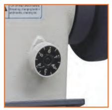
Fig 2.2.21: Reverse feed lever
