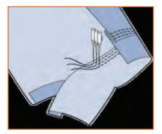
**Lap Felled Seam:** The Lap Felled type, involves only one stitching operation - a strong seam with fabric edges protected from fraying. Commonly used for making up jeans or similar garments.
