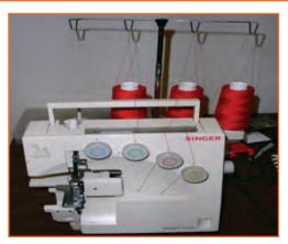
Fig 2.2.6: Three Thread Overlock Machine
