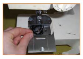
**Step 9:** Pull the string out tight and set the bobbin into the tray. Insert the thread into the metal notch and pull back.
