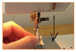
Step 2: Remove the needle by pulling down and away from the needle clamp.
