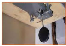
**Knee Lifter:** is used to lift the presser foot with the use of knee. **Hand Lifter:** is used to lift the presser foot.
