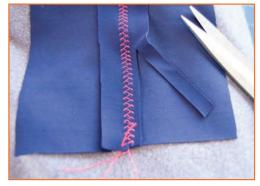
Fig 2.2.10: Multi-Thread Flat Lock
