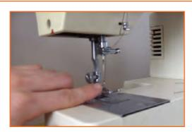
**Step 7:** Then thread the needle front to back or right to left depending on your machine. Pull enough thread through so that it does not pull out when the needle moves 5-10 inches.
