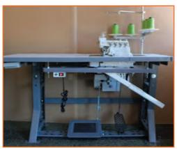
**Four Thread Overlock Machine:** This machine stitches a chain stitch or a safety stitch and overcasts seams. Four-thread overlock machine has two needles and two loopers and this can be converted to both two and three thread overlock. All 4 threads are necessary to sew a serged seam. This type of machine is used for sewing blouses, shirts, skirts, dresses, pants, lingerie, action wear, swimwear, and even sleepwear.
