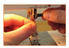
Step 4: Use your fingers initially and then your tool of choice to tighten the needle clamp screw. The tighter you can make this, the better. A loose clamp may leave the needle down in the fabric you are sewing.
