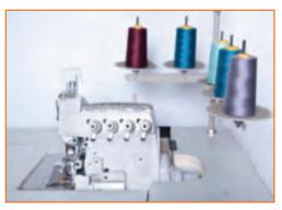
Fig 2.2.8(a): Five-Thread Overlock Machine
