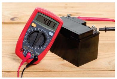
Fig. 1.1.5: Measurement of DC voltage
