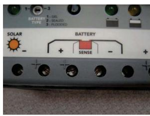
Fig. 2.3.8: Battery voltage sensing of a charge controller
