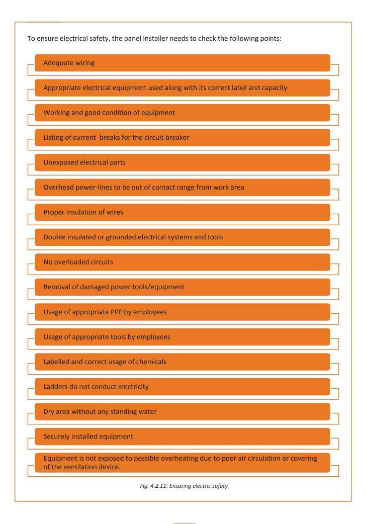
Some electrical safety points while installation and maintenance of a PV system are mentioned in the following figure:
