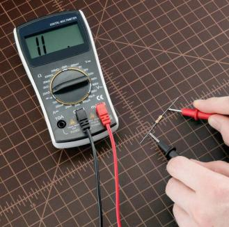
Fig. 1.1.7: Measurement of resistance
