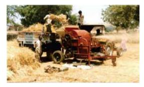
Fig 1.1.1 High capacity multi-crop thresher
