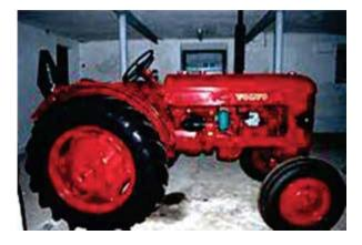
Fig 1.2.1 Volvo T25, 1956, gasoline tractor
