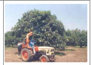
Fig 1.5.1 Aero Blast Orchard Sprayer
