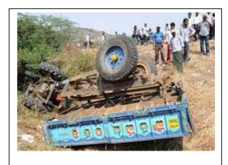
Fig 4.3.1 Accident caused due to absence of braking system in trailer
