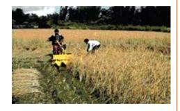
Fig 1.1.1 Self-propelled walking type vertical conveyor reaper
