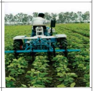
Fig 1.5.1 Three-row rotary weeder
