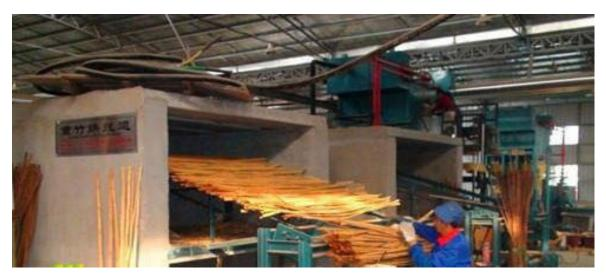
• STEP 3: Combine the bamboo sliver in the form of common lot and feed it to the dryer machine. This procedure takes relatively lesser time than fire method.
