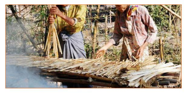
• STEP 2: Place the bamboo slivers on a rack and dry the bamboo sliver using fire under it at appropriate distance. This procedure takes relatively lesser time than open air procedure.
