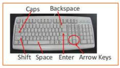
Fig.10.2.2: Parts of a Keyboard
