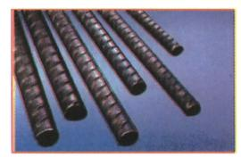
Fig 5.1.1: Reinforcement bars
