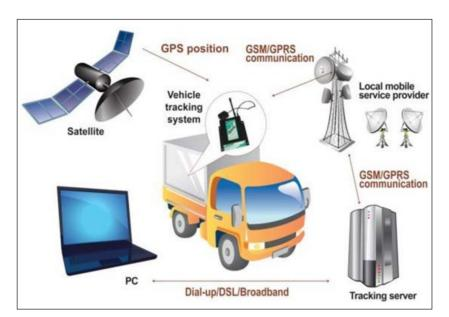
Fig 5.1 - GPS Tracking System
