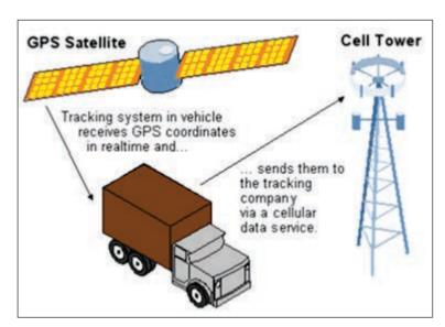
Fig 3.4 - GPS tracking System
