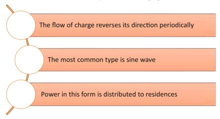
Fig 2.2.2: Features of alternating current
