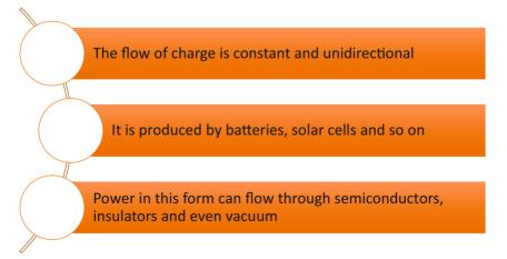
Fig 2.2.3: Features of direct current
