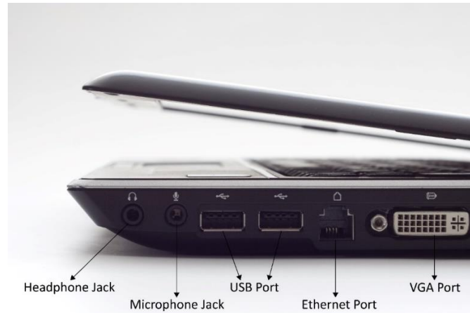
Fig. 4.1.7: Different connection ports in a laptop computer
