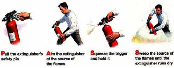
Fig 2.4.2: Using fire extinguisher
