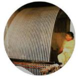
**Warping**. The twist is comprised of cotton strings (yarn) organized lengthwise, extended on the loom towards the weaver. To make the twist, yarn is twisted to the required length on a warping wheel.
