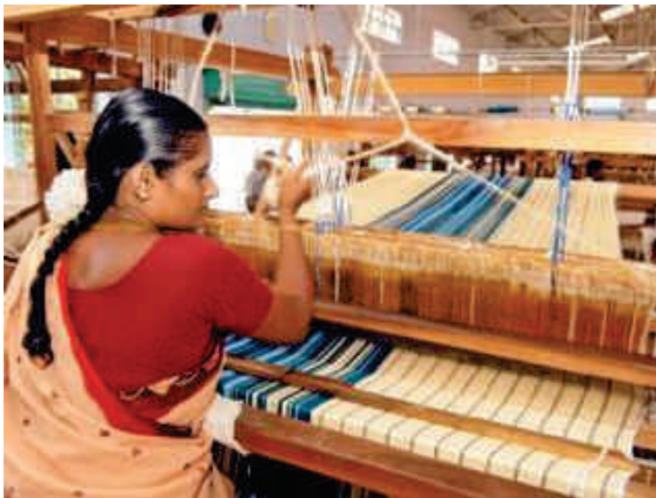
Figure 3.1. 1A Simple Handloom
