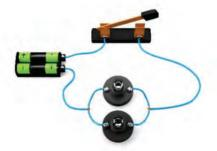
Fig 1.26: Connec on of lamp in parallel
