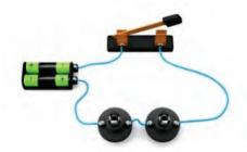
Fig 1.25: Connec on of lamp in series
