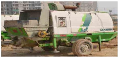
Fig. 4.2.3. Concrete Pump
