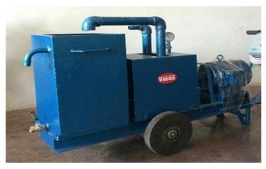
Fig. 4.2.7. Vacuum De-watering Machine
