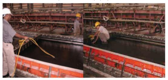
Fig.4.4.9. Cleaning Mould and applying the oil/mould release agents
