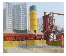
Fig. 1.3.5.Batching Plant for concrete mixing
