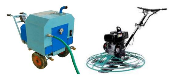
Fig. 5.3.2. Power tools for Tremix Flooring
