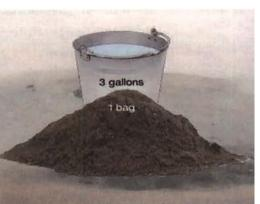
Fig 5.3.6: Mixing of mortar and water
