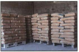
Fig 5.3.7: Stacking of cement bags
