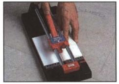
Fig 5.2.7: Inserting tile in the machine
