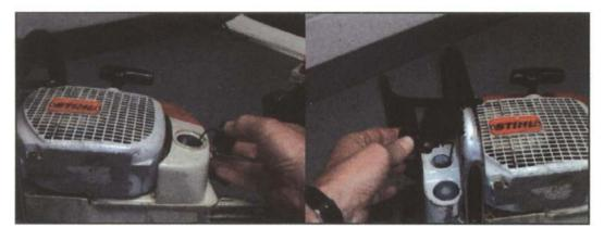
Fig 4.1.16: Power saw lubrication
