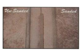
Fig 4.2.9: Non-sanded and sanded grout
