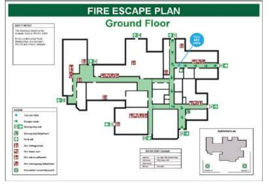
Fig. 15.6.1: Diagram of a fire escape route (image courtesy: https://www.Visualbuilding.Co.Uk)
