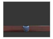
Fig. 6.1.2.7 - Excessive Penetration
