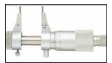
Fig. 0.5.2.9 - Inside Micrometer
