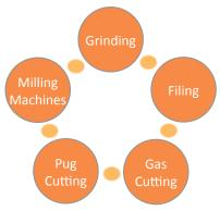
Fig. 4.5.2 - Methods of Edge Preparation
